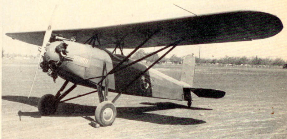
Final production model of the Inland line was the R-400 Sportster with a 90-hp Warner Scarab Jr. Later refinements like steerable tailwheel, low-pressure tires, and conveniences like an electric starter couldn't help sales in the face of the depression.
